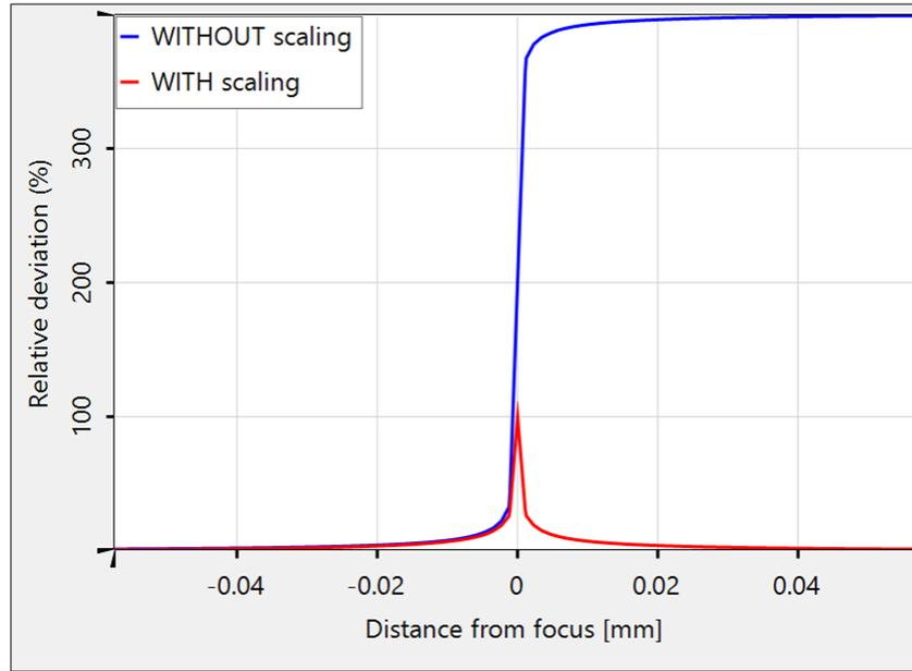
Figure 2: The figure shows a plot of the relative standard deviation (Eq. 1) of the geometrically propagated field with respect to the same field propagated with SPW. For the blue curve the geometric and the diffractive results were compared as-is, for the red curve the geometric result was multiplied by a constant  $\gamma(z_i) \in \mathbb{C}$  which minimises the value of  $\sigma$ .
