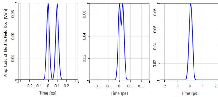
Figure 4: Second Harmonic in time domain with pulse lengths of 35 fs, 100 fs and 250 fs. The splitting effect disappears at higher lengths as it is overlaid by the temporal broadness of the second harmonic.
