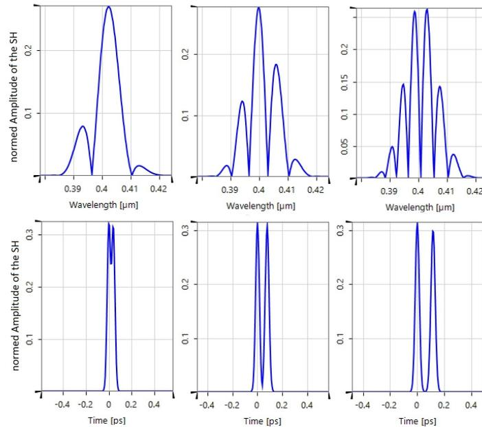
Figure 3: Second harmonic at various crystal lengths in the non-phase-matched case. The angle is 26 and the nonlinear material BBO. The destructive interference is resulting in an filtering of certain frequencies depending on the length of the crystal.
