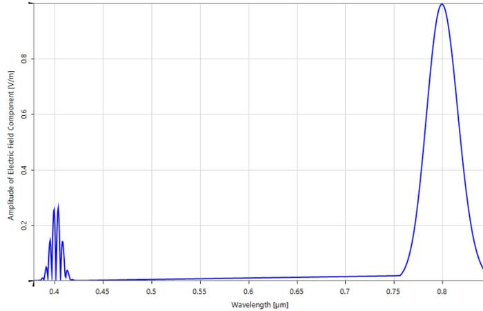
Figure 2: Fundamental pulse and second harmonic for BBO after 700  $\mu\text{m}$ . In this simulation we assumed an incident angle of  $26^\circ$ . Even small derivations from the phase-matching angle lead to an enormous decrease of the amplitude of the second harmonic in comparison to the fundamental pulse.
