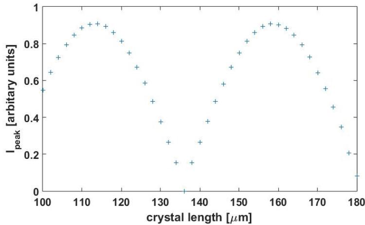
Figure 1: Peak Amplitude of a monochromatic 800 nm light shown over different crystal lengths. The coherence length is about  $40 \mu\text{m}$ .
